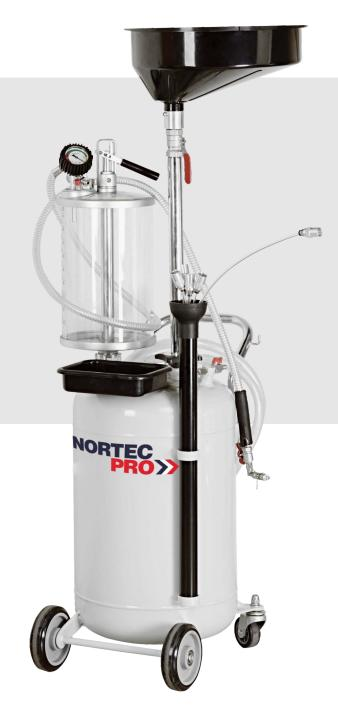
TANK CAPACITY: 90L CONTROL TANK CAPACITY: 8L 65-70L CAPACITY TO FILL WITH LIOUID: **VACUUM AIR PRESSURE:** 7-8 BAR 150-180\$ SEALING TIME: SUCTION EFFICIENCY: 1,5-2L/MIN LW. SUCTION CABLE: 2000 MM SPINDLE BOWL CAPACITY: 18L **CUP DIAMETER:** 400MM 1700MM MAX HEIGHT OF THE SINK BOWL: MIN. HEIGHT OF SINK BOWL: 100MM MAX. MOLD VOLUME: 70L MAX.GUMING PRESSURE: 1BAR LW. DRAIN PIPE: 2000MM AIR INLET FITTING: 1/4" QUICK COUPLER: 1/4" NPT FEMALE WEIGHT: 43 KG
