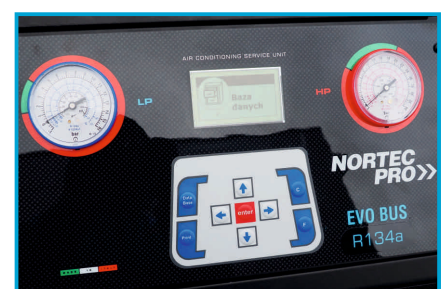
CLEAR CONTROL PANEL
