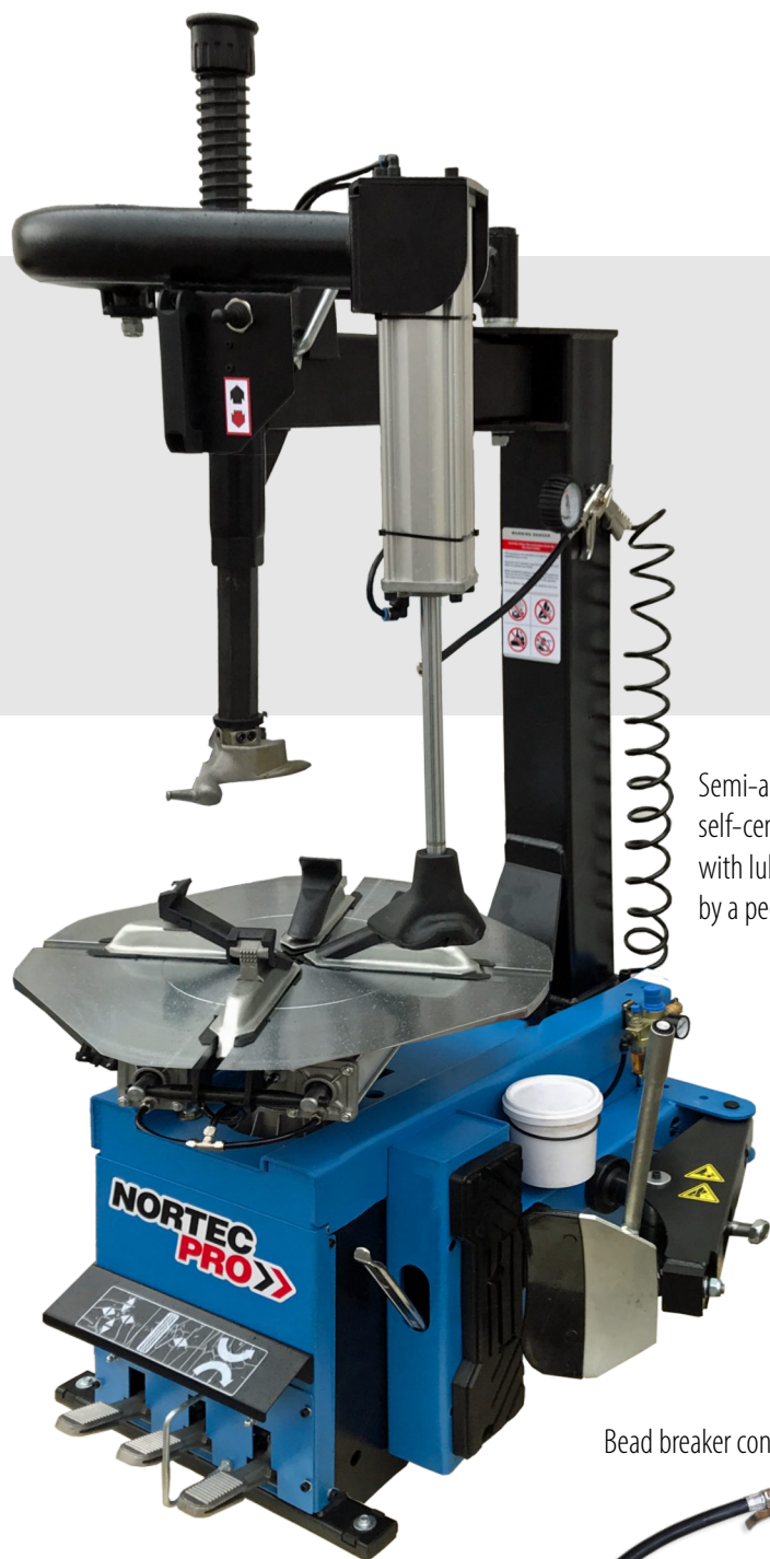
Rotating arm with pneumatic bead pushing device
